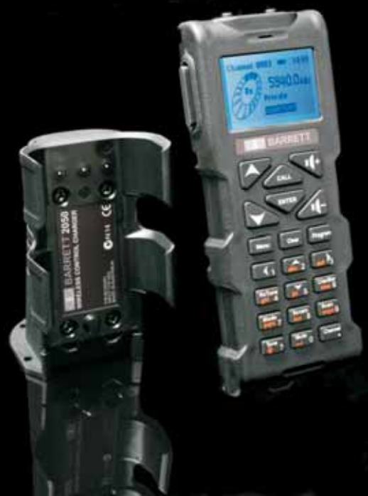
The handset mounting cradle, which also charges the battery, separates to allow mounting on the top or the front of dashboards
